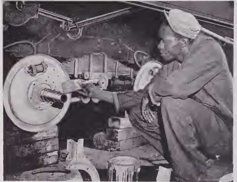
FIGURE 2. To minimize salt water corrosion, brake mechanisms and wheel backing plates are painted with zinc chromate and Rust Preventive Thin Film at Oahu DUKW school.
